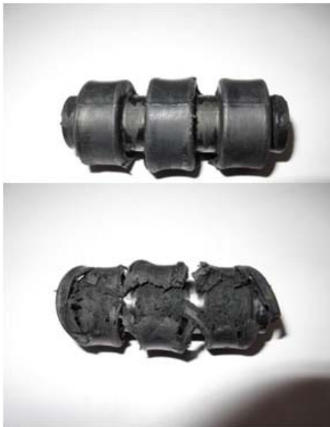
Figure 4: MIL-DTL-11891 T130 Bushing Failure
