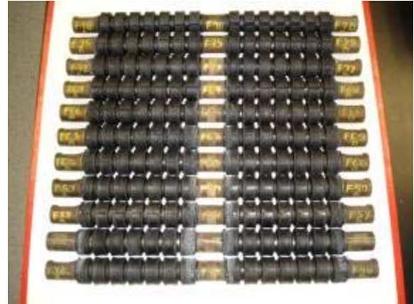
Figure 5: Progression of Bushing Failures (Top new bushings, bottom worn bushings, 250 mile increments between samples)
