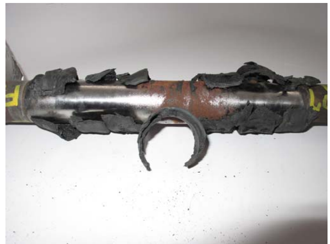
Figure 6: T158LL Bushing Failures
