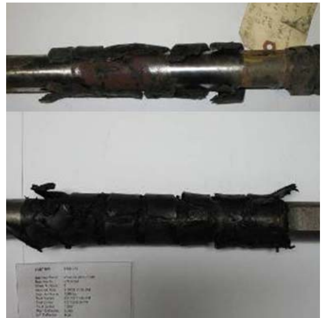
Figure 9: Radial and Torsional Failure from Field (top) and Lab Test (bottom)
